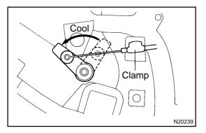
(b) Adjust air mix control cable.Set the cable connector to air mix link pin on left side of A/C unit and clamp the cable outer on condition.
