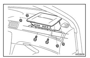
Remove the 2 bolts, 4 nuts and front passenger airbag assembly.
