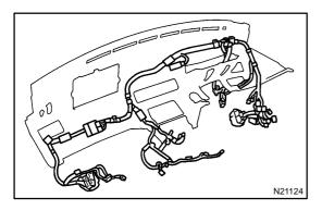
2. REMOVE INSTRUMENT PANEL WIRE HARNESS Remove the 2 brackets, 8 clips and wire harness.
