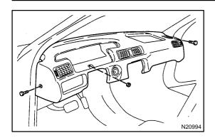
(f) Remove the bolt, nut, screw and the instrument panel assembly.
