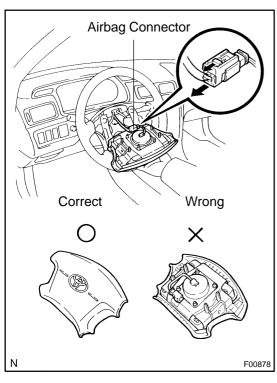
(d) Pull the pad out from the steering wheel and disconnect the airbag connector.
